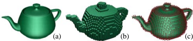
Figure 3. Teapot: (a) polygonal model, (b) voxel model, (c) point shell model.
