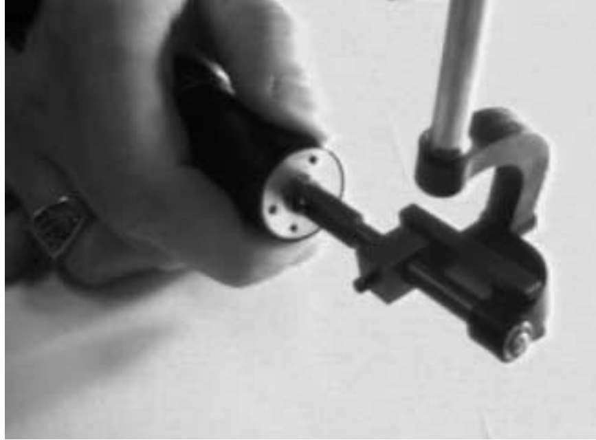
Figure 4-1: A 1 degree-of-freedom active screwdriver for driving virtual screws
